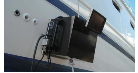
真空负压加载罩 Vacuum Hood
